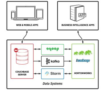
For use cases where batch import/export between Couchbase Server and Hadoop makes sense, the Sqoop plugin can be utilized to transfer data between Couchbase Server and HDP. It leverages map/reduce to import and export data via parallel tasks. It enables enterprises to export operational data from Couchbase Server to HDP for offline analytics and processing, and to import processed data from HDP into Couchbase Server to improve operational efficiency.
